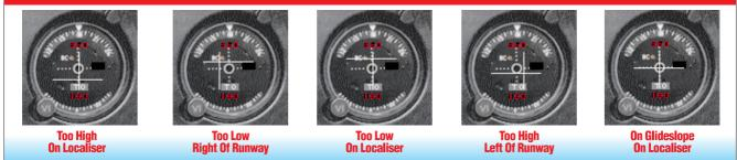
Above: The ILS receiver in the aircraft. The vertical needle is the localiser, the horizontal needle is the glideslope. The circle in the centre is your aircraft. The aim is to is to centre the needles in the circle as illustrated on the far right.
